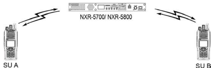
Figure 12-1 Single Repeater System
