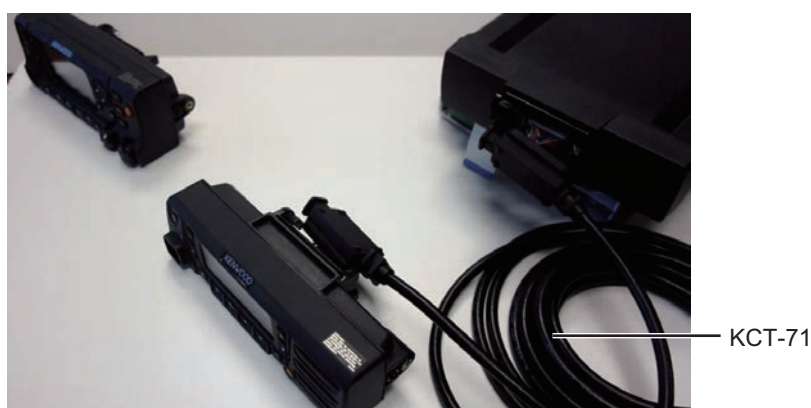
Figure 18-8 Connection of the KCT-71 Cables
