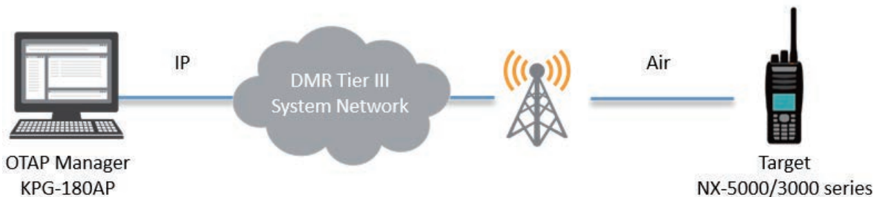
Figure 3-8 IP Connection by the IP Based Packet Data Format
