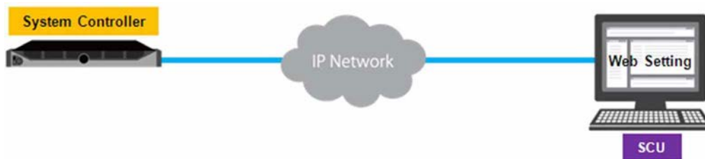
Figure 1-1 Connecting to SCU
