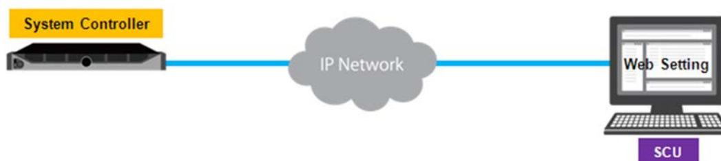
Figure 3-13 Connecting to SCU
